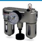
The FRL-15 is a combination air filter/regulator/lubricator unit that controls the air pressure to the chuck's built-in cylinder, and provides lubrication to the rotary air bearing assembly. This unit also filters contaminants from the air supply. Water that accumulates in the filter unit can be purged by a manual drain.
