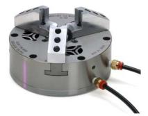
Stationary air chucks are ideal for milling, drilling, tapping, and other applications requiring a compact self-contained workholding fixture. Air is supplied directly into the side of the chuck body, and the chuck can be mounted directly to the machine table or pallet. Through holes are available on all models.
