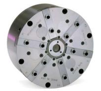
Large Diameter Air Chucks offer high accuracy and adjustable clamping force for machining large diameter precision and thin-walled workpieces. Large Diameter chucks are available in three jaw as well as two and six jaw configurations. Large Diameter models with extended jaw stroke, air ports on OD of chuck body for stationary applications, and other special configurations are quoted upon request.
