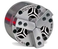
Rotating air chucks are ideal for precision turning and cylindrical grinding applications that require close concentricity, squareness, and parallelism tolerances. Variable clamping force enables clamping of thin-walled and other fragile parts with minimal distortion. All models, except the 3-50, feature a coolant or air passage through the center of the chuck.
