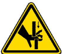
**Always make sure to keep your hands and fingers clear of the top jaws and workpiece as the chuck is clamped.**
