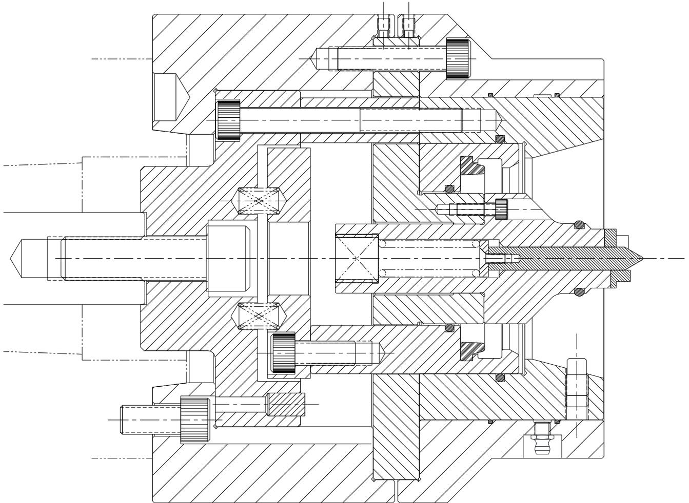
1. With a test indicator, ensure the runout of the ID of the driver mounting plate is within .0002, as shown in Step 8.2B. If runout is not within .0002, remove chuck body and return to Step 8.2B.
