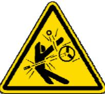
**Do not exceed maximum recommended speed of the chuck for a given input pressure.**
