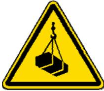
**Always lift the chuck by using an eyebolt or lifting belt, and stand clear of suspended loads.**
