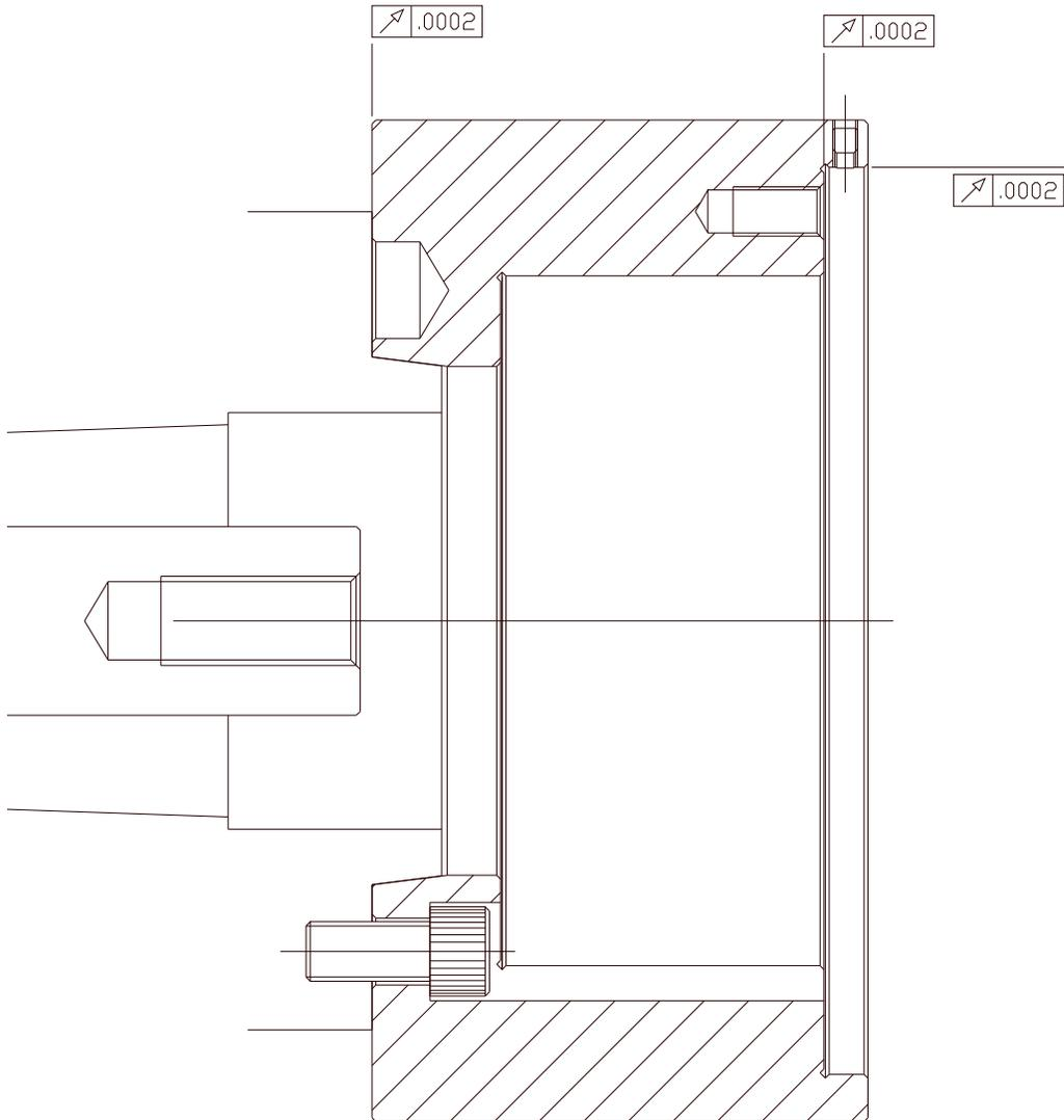
1. Make certain that the mounting faces of the machine spindle and the adapter plate are free of nicks, burrs, or foreign material that could prevent proper seating.
