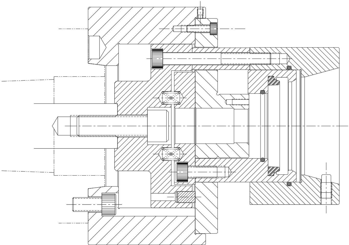
1. Actuate the hydraulic cylinder using minimal cylinder pressure to fully extend the draw bar.
