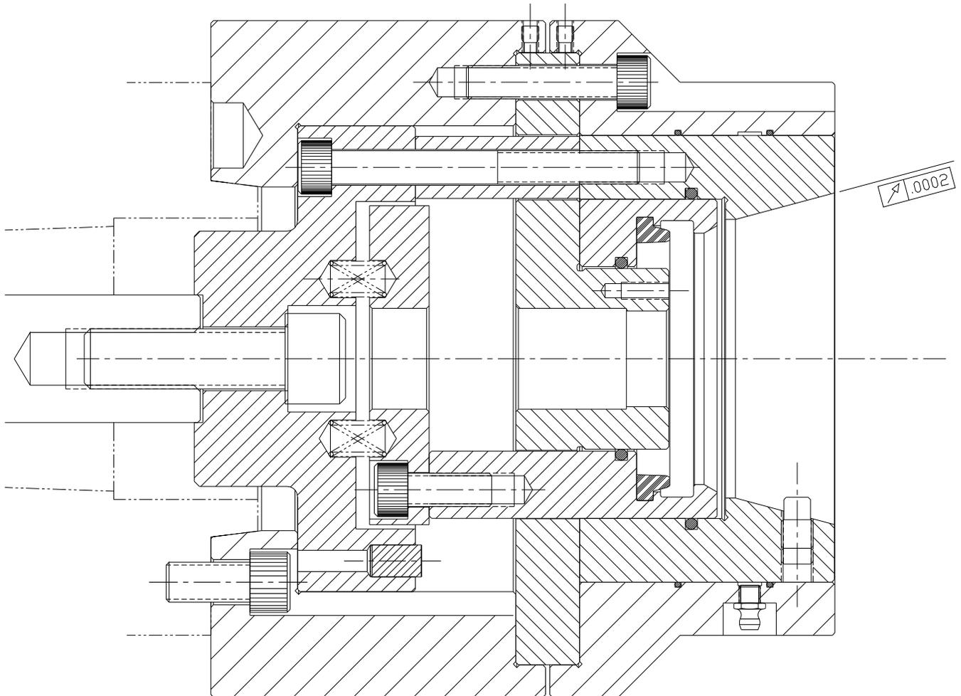
1. Install chuck body over chuck assembly and lightly tighten mounting screws.
